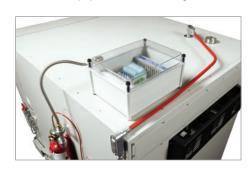
This safety option is designed to control a fire by displacing oxygen and applying a cooling effect directly to the product being tested.
