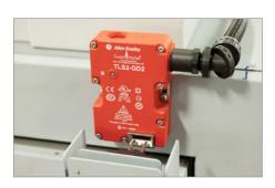
Prevents access to the testing chamber during a normal cycle or when an alarm condition has been detected.
