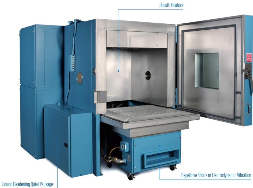
A Thermotron AGREE Chamber provides the flexibility to adapt to ever-changing test requirements.
