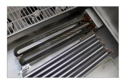
Sheath heaters provide high reliability and peace of mind as they safely limit the temperature.
